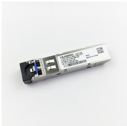
Transeiver ottico Huawei S-SFP-GE-LH80-SM1550, eSFP, GE, modulo monomodale (1550 nm, 80 km, LC)
