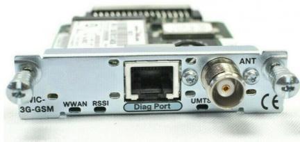
Cisco HWIC-3G-GSM 3G WWAN HWIC-HSDPA/UMTS/EDGE/GPRS-850/900/2100MHz
