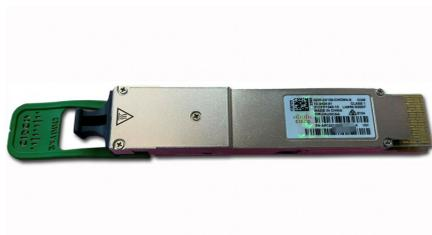
Ricetrasmittitore Cisco QDD-2X100-CWDM4-S 2X 100G QSFP-DD, 2X 100G-CWDM4, Dual Duplex CS, 2 km Duplex SMF
