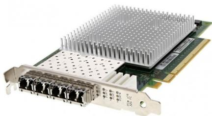
Originale Qlogic QLE2764-SR-CK PCIe 3.0 x16 Quad-port 32GFC SR-Optic SFP+ 32Gb Fibre Channel Adapter
