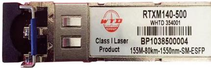
Modulo transceiver ottico WTD RTX140-500 155M 80km 1550nm SM ESFP
