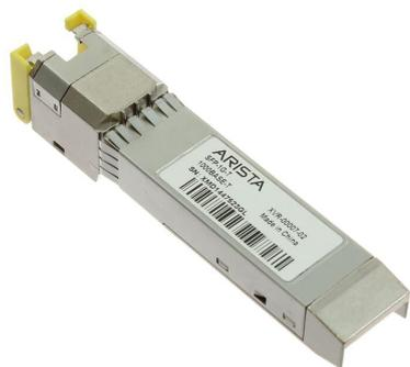
Arista SFP-1G-T XVR-00007-02 Ricetrasmittitore in rame 100/1000BASE-T SFP
